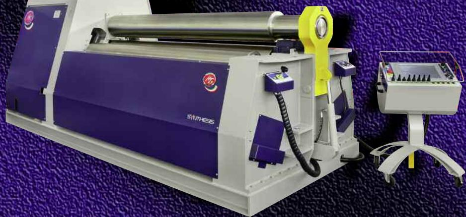
3-roll plate bending machines, for sheet thickness from 1 mm up to 300 mm, very easy to operate. **G** with planetary side roll system and parallelism controlled by torsion bars, **GE** with electronic parallelism, **GL** Electronic parallelism and side rolls moving on linear guides.
