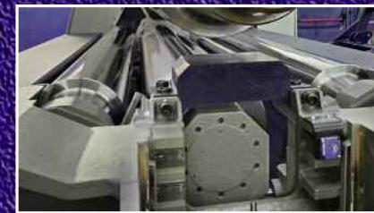
Variable geometry 3-roll plate bending machines, for sheet thickness from 20 mm up to 300 mm. These MG machines ensure the best combination of rolling power and precision when pre-bending heavy materials.
